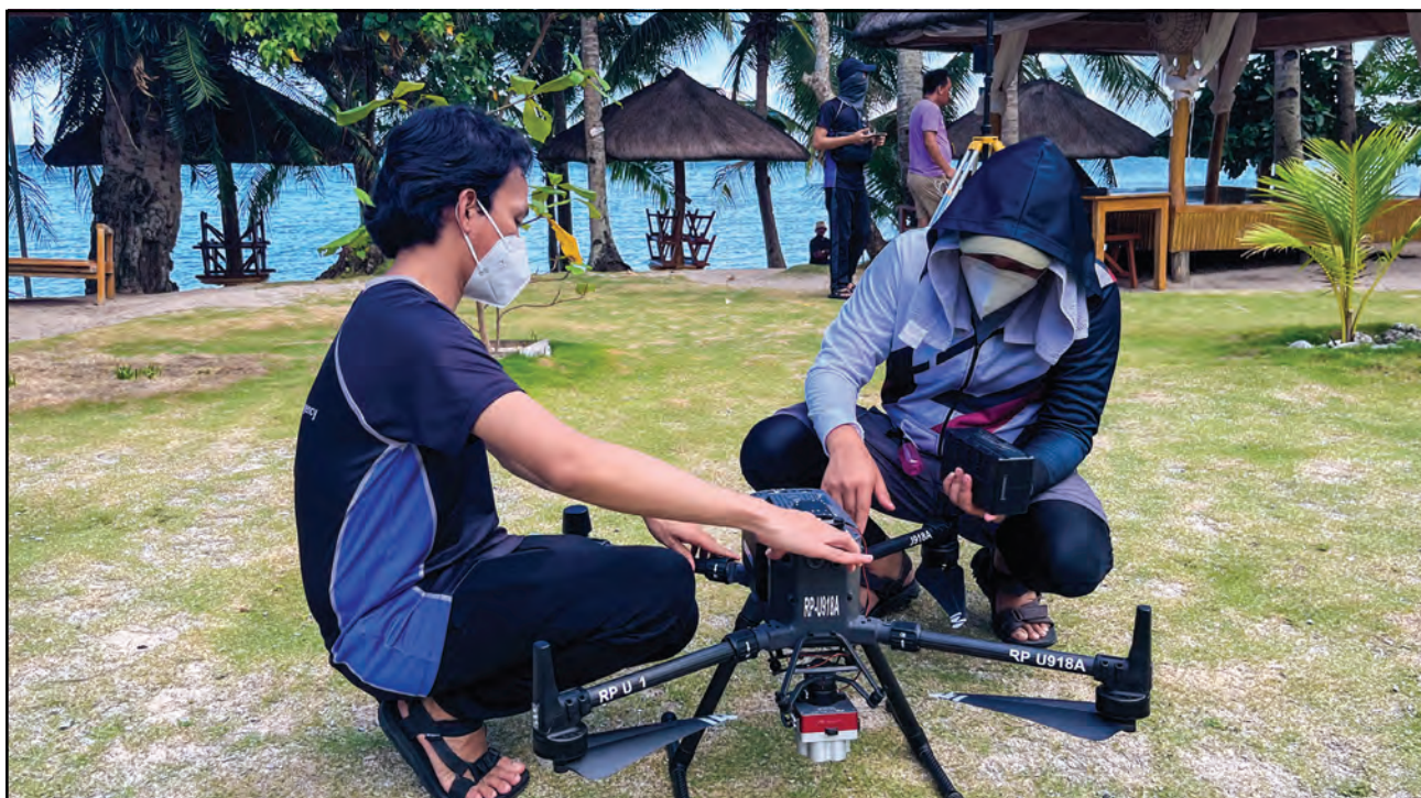
PhilSA personnel utilizes drone technology to validate benthic maps (e.g., corals, seagrass, etc.) and mangrove maps extracted from satellite data. These maps are integral in monitoring and assessing the status and conditions of ecosystems.
